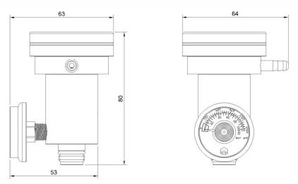
The Demand Flow Regulator-C10 is used for calibration gases, pump based instruments and handheld gas detectors. These regulators supply gas as demanded by the instrument and automatically shuts off.
